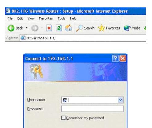
In order to configure the Wireless 11g AP Router, you must enter the password into the **Password** box and leave the **User Name** blank. The default password is "**admin**".
